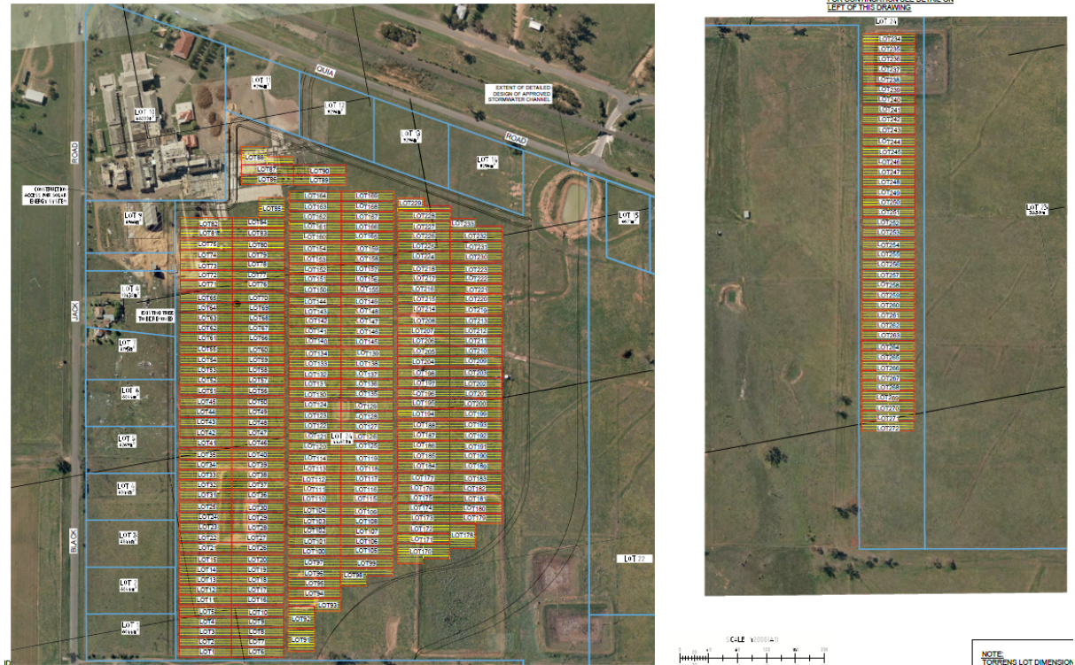
Figure 2 – Solar Array Set out
